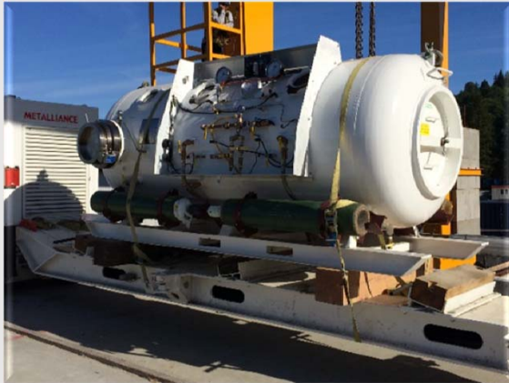
Transfer Lock on MSV
